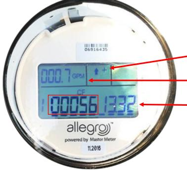
The billed consumption is calculated by subtracting the reading taken at the start of the billing period from the reading taken at the end of the billing period. Using the examples above, 1.00 billing Units subtracted from 56.00 billing Units is 55.00 billing Units.
