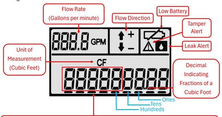
The third through seventh digits to the left of the decimal point show the total billing units measured since the register was installed, or since your last monthly bill reading.
